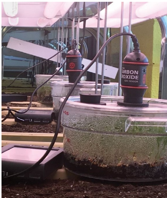
Figure 5. Students experiment with sealed environments by monitoring carbon dioxide levels over a three-week period to document levels as seeds germinate using cellular respiration and then begin to utilize photosynthesis.
