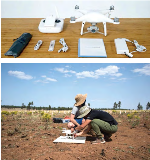
Figure 5A. (top) DJI Phantom 4 drone and components used for aerial imagery and site surveying. Photo credit: John Fegyveresi
