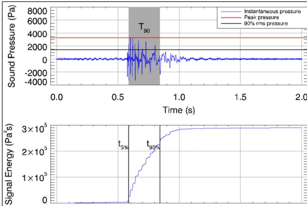
**Figure A-2. The rms90 value is computed using the rms square pressure over  $T_{90}$ , the period between the time of 5% and 95% of the cumulative square pressure**
