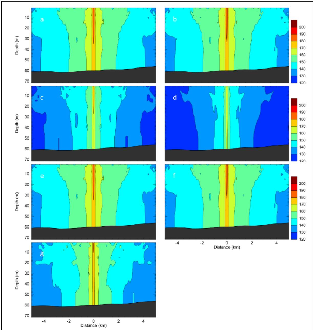
**Figure 6. Knudsen 320 B/R 3.5 kHz sound exposure level at the Atlantic (24.5390°N, -80.7623°E) modeling site in mid-depth water. a) Unweighted b) LF weighted c) MF weighted d) HF weighted e) OPW weighted f) PPW weighted g) SI weighted.**
