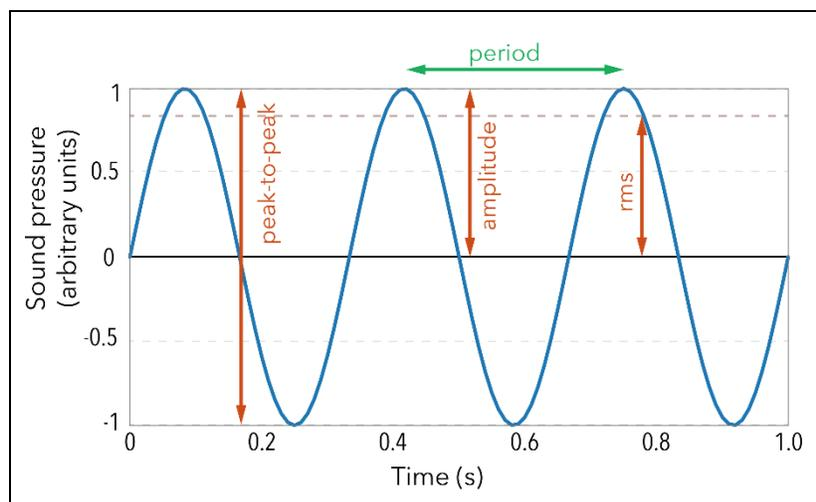
**Figure A-1. A cosine wave with a peak value (i.e., amplitude) of 1, peak-to-peak value of 2, rms value of 0.71, period of 0.33 s, and frequency of 3 Hz.**
