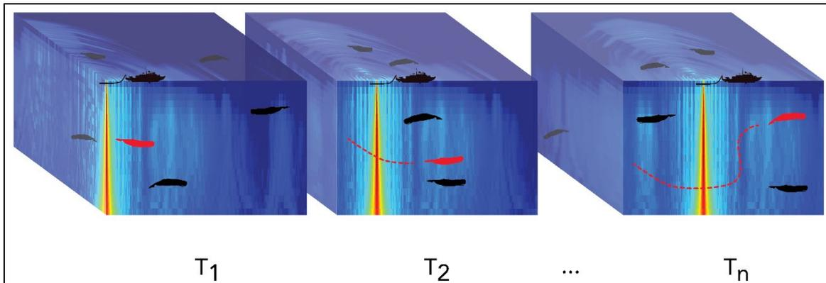
**Figure C-4. Graphic of animats in a moving sound field. Example animat (red) shown moving with each time step. The acoustic exposure of each animat is determined by where it is in the sound field, and its exposure history is accumulated as the simulation steps through time.**
