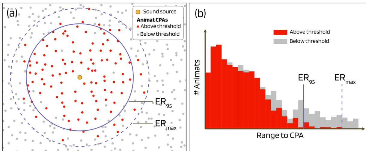
**Figure 3. Example distribution of animat closest points of approach (CPAs). Panel (a) shows the horizontal distribution of animats near a sound source. Panel (b) shows the distribution of ranges to animat CPAs. The 95% and maximum Exposure Ranges (ER<sub>95%</sub> and ER<sub>max</sub>) are indicated in both panels.**
