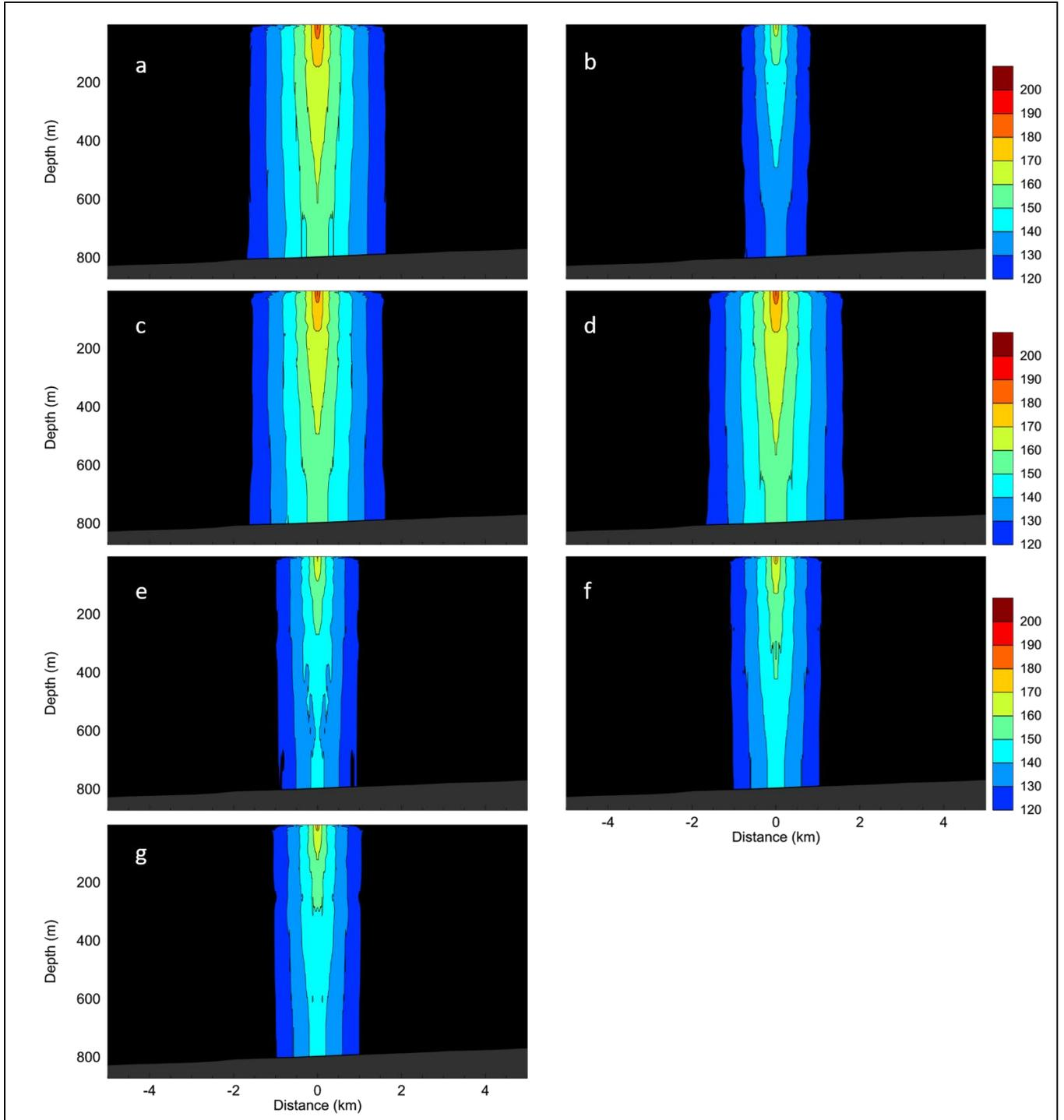
Figure 5. Kongsberg EM710 at 70 kHz sound exposure level at the Atlantic (24.821°N, -79.9265°E) modeling site in deep water. a) Unweighted b) LF weighted c) MF weighted d) HF weighted e) OPW weighted f) PPW weighted g) SI weighted.
