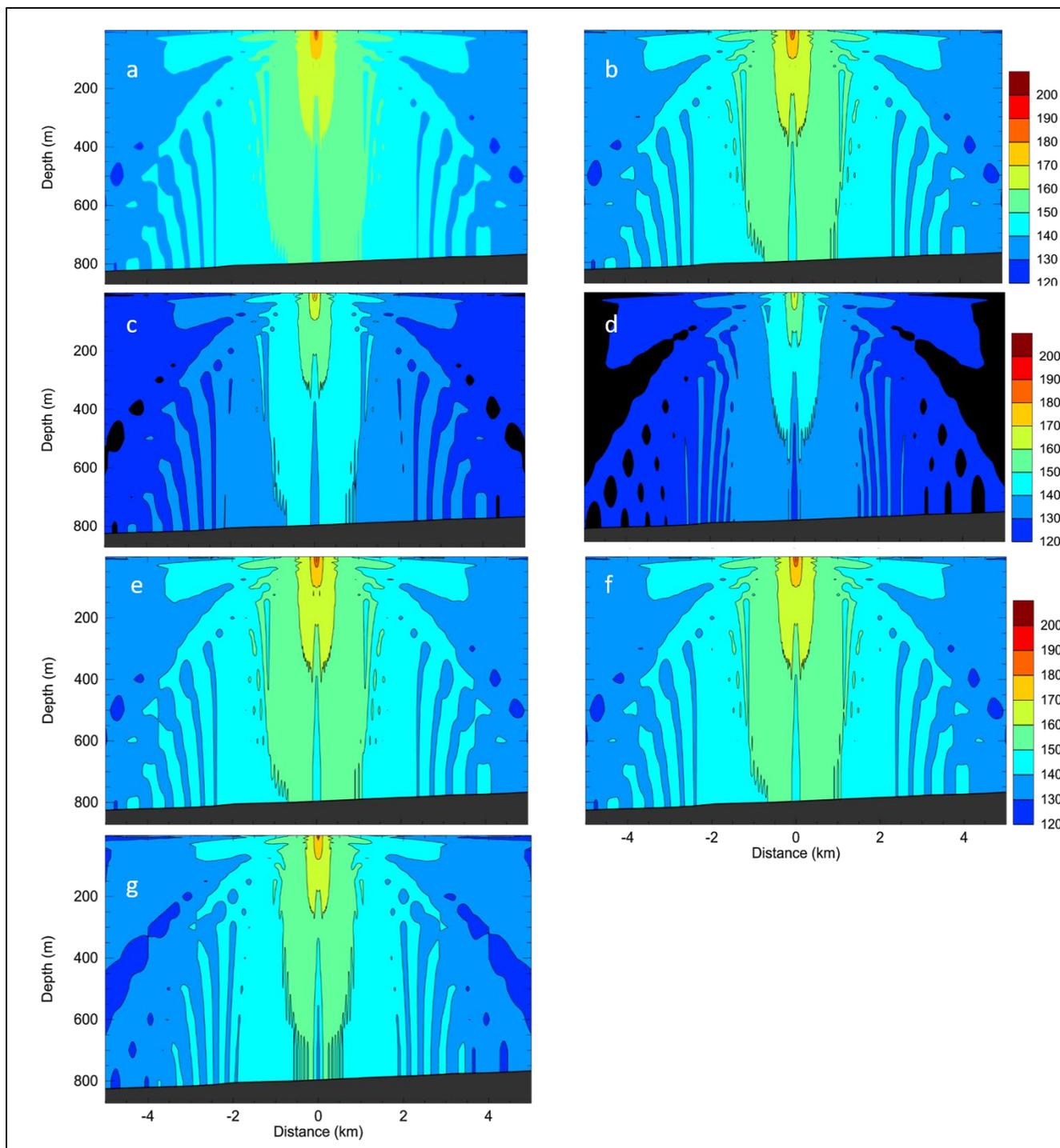
Figure 4. Knudsen 320 B/R 3.5 kHz sound exposure level at the Atlantic (24.821°N, -79.9265°E) modeling site in deep water. a) Unweighted b) LF weighted c) MF weighted d) HF weighted e) OPW weighted f) PPW weighted g) SI weighted.
