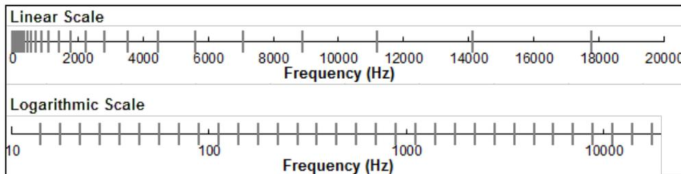
**Figure A-3. Decidecade frequency bands (vertical lines) shown on a linear frequency scale and a logarithmic scale**
