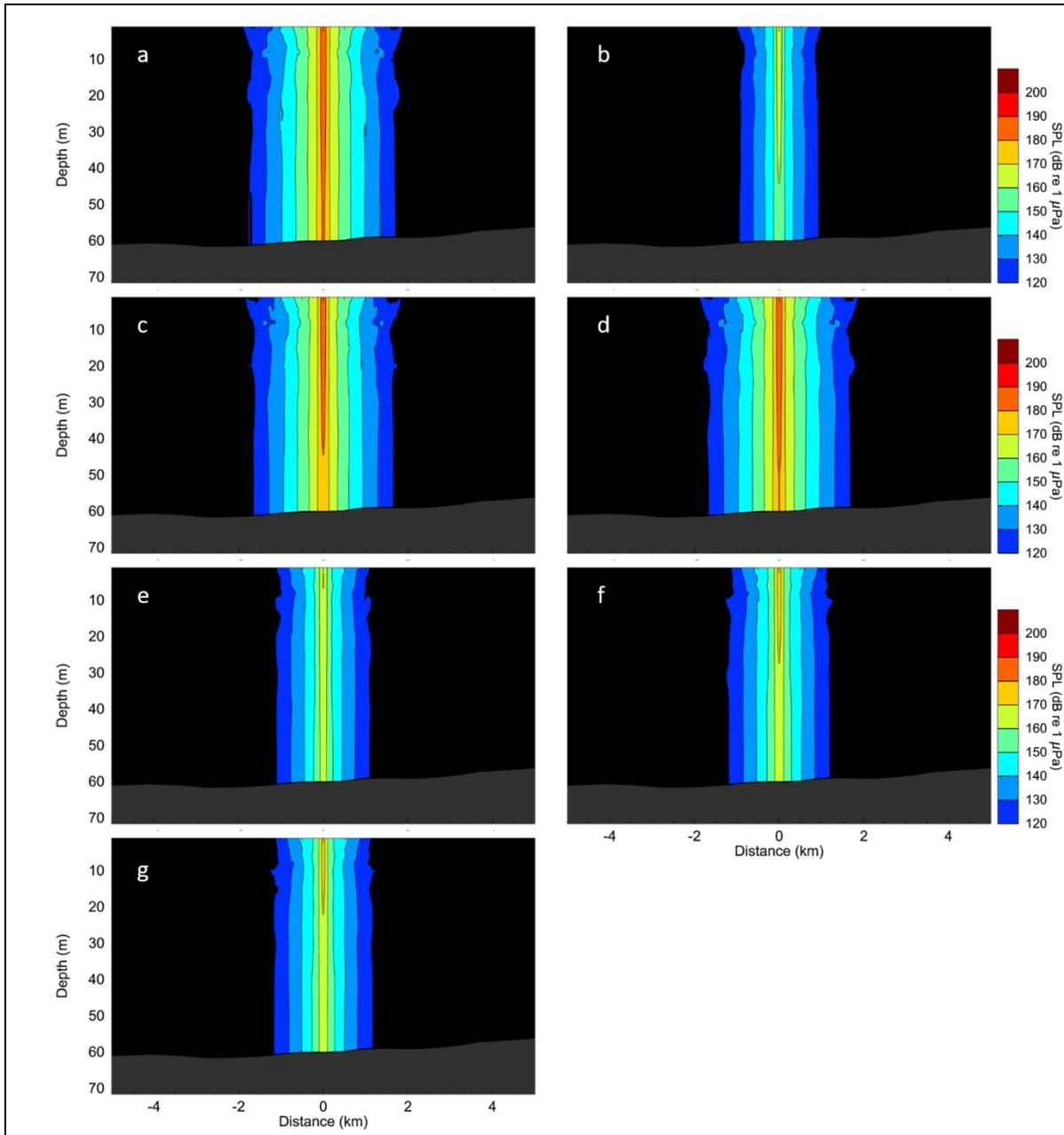
**Figure 7. Kongsberg EM710 at 70 kHz sound exposure level at the Atlantic (24.5390°N, -80.7623°E) modeling site in mid-depth water. a) Unweighted b) LF weighted c) MF weighted d) HF weighted e) OPW weighted f) PPW weighted g) SI weighted.**
