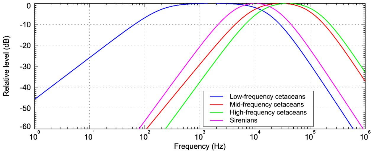
**Figure B-3. Auditory weighting functions for the low-, mid-, and high-frequency cetacean and sirenian hearing groups as recommended by NMFS (2018). Sirenian weighting function is from Blackstock et al. (2017)**
