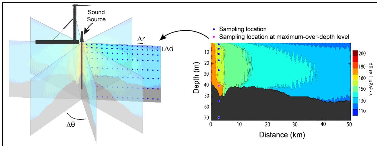
**Figure C-2. Modeled three-dimensional sound field (N×2-D method) and maximum-over-depth modeling approach. Sampling locations are shown as blue dots on both figures. On the right panel, the pink dot represents the sampling location where the sound level is maximum over the water column. This maximum-over-depth level is used in calculating distances to sound level thresholds for some marine animals.**
