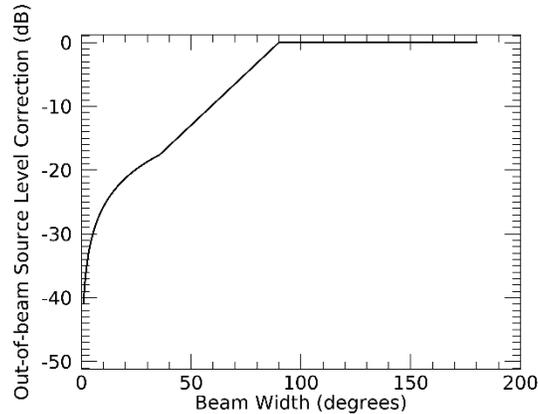
**Figure C-1. Correction for calculating out-of-beam source level (i.e., in the horizontal direction) from in-beam source level, as a function of source beamwidth.**
