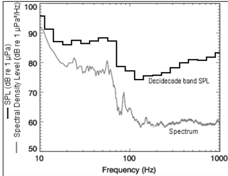
**Figure A-4. Sound pressure spectral density levels and the corresponding decidecade band sound pressure levels of example ambient noise shown on a logarithmic frequency scale**
