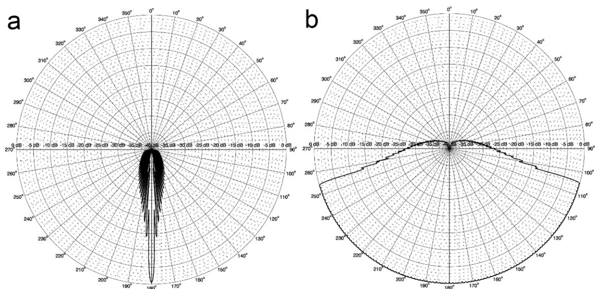
**Figure 1. Vertical slice for the Modelled beam pattern for a multibeam system with 191 individual 2°x2° beams, making a 150° swath perpendicular to the vessel track; (a) along- and (b) across-track direction.**
