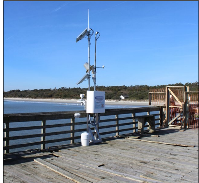
Figure 3.11-4. Tide Gauge on a Pier
